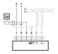
Switching contact requirements: The switching contact must be able to switch a current of 16 mA at 24V accurately.
